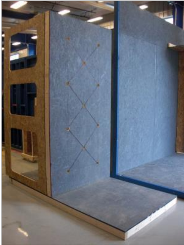
A self standing Task Wall can be fabricated by teams or assembled into the DRC Trial Stage (with additional signage header over top and optional terrain in front)
